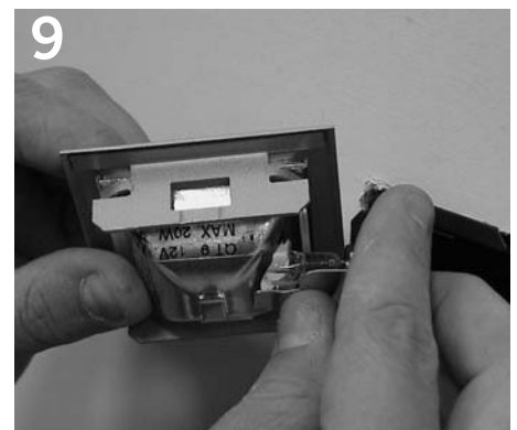
9 Slide lamp and lamp socket into reflector assembly.
