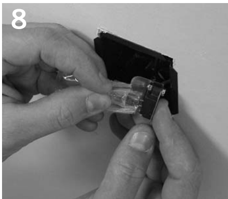
8 Install lamp per relamp label. NOTE: Lamp should not be touched with bare hand.
