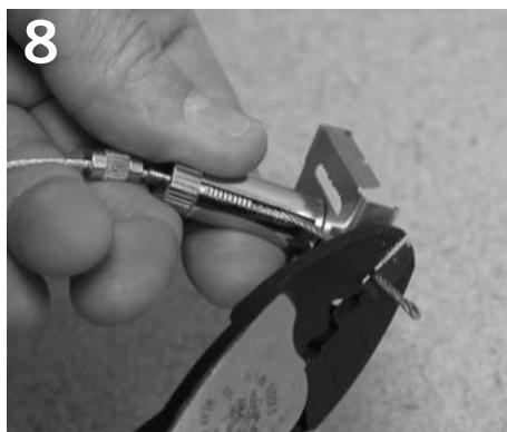
Trim excess cables with wire-cutter.
