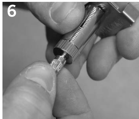
6 Unscrew gripper button cover.
