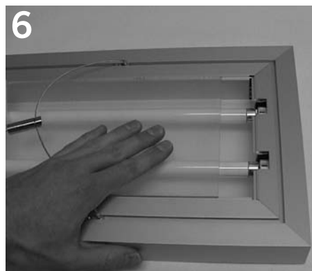
Secure clear acrylic top cover into place.
