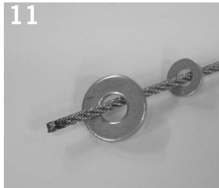
11 Place large washers on suspension cables - one per cable.
