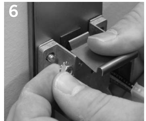
6 Secure mounting bracket with nuts.
