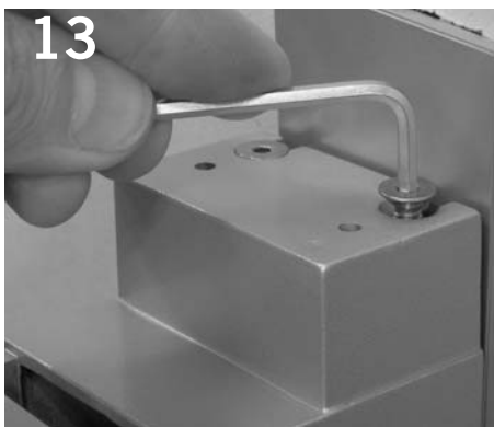
13 Secure fixture with screws as shown.
