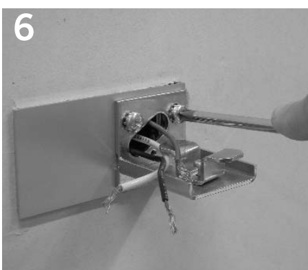
6 Install support bracket and trim plate to mounting plate using (2) M5 x 8mm screws with lock washers (provided). Level bracket and tighten screws. Route leads through opening in bracket.
