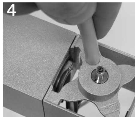
4 Insert feed cord until jacket is inside cord opening in end block.
