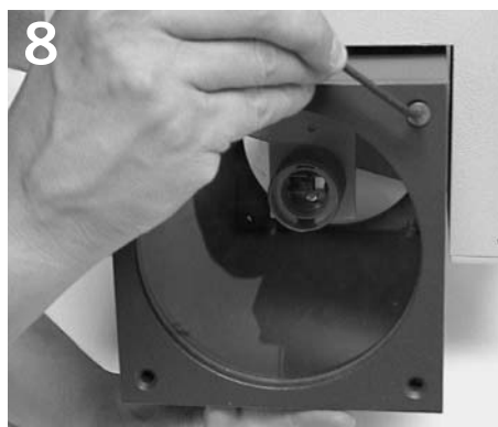
8 Remove lamp coverplates with hex wrench.
