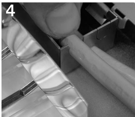
4 Seat cord into void left from tab removal. NOTE: Cord must be properly seated for replacement of splice compartment cover.
