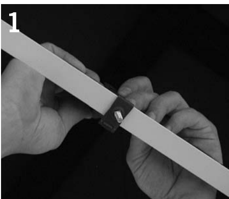
1 Fasten caddy clip around spline.
