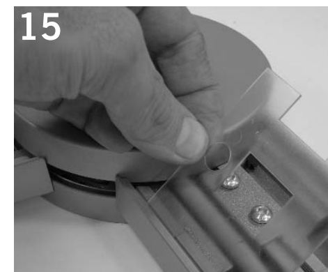
15 Install clear plastic node coupler covers, as shown.
