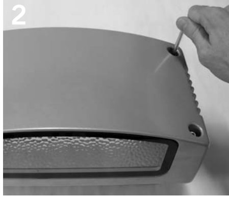
2 Loosen (4) corner screws with wrench provided (5.0mm hex).
