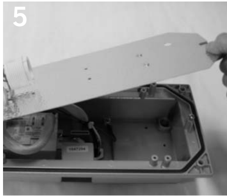
5 Slide reflector to one side and lift away from lower housing. Reflector will remain tethered via wiring.
