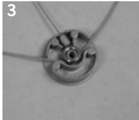
3 Lay swaged end of long cable into adjuster button and reassemble button.
