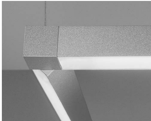
Rotation at the corners is limited. One lighting element must be in the 0°, 90°, 180° or 270° position to enable the other lighting element to rotate through the entire 360° range.
