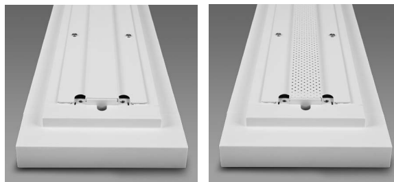
Perforated or solid top are available to change the uplight/downlight percentage.
